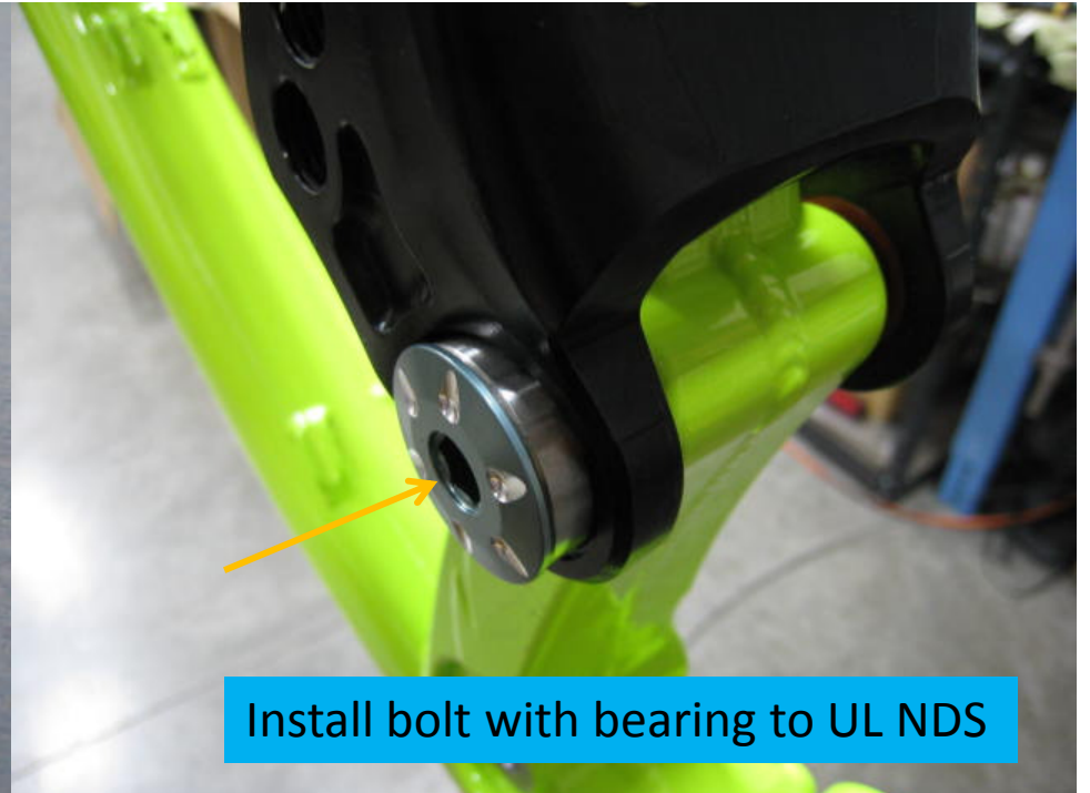
Torque bolts to 35NM
