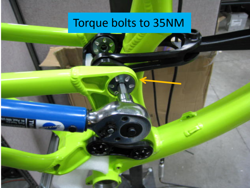
Apply blue loctite 243to Threads in UL
