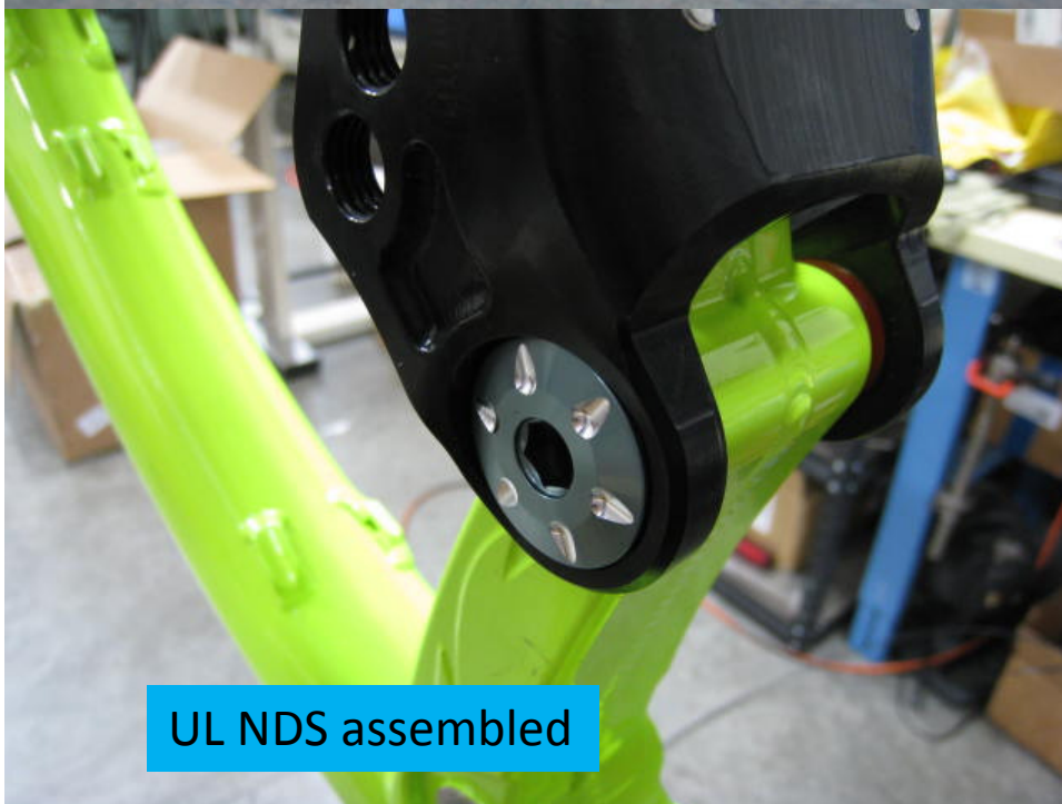
M14 bolt and bearing
